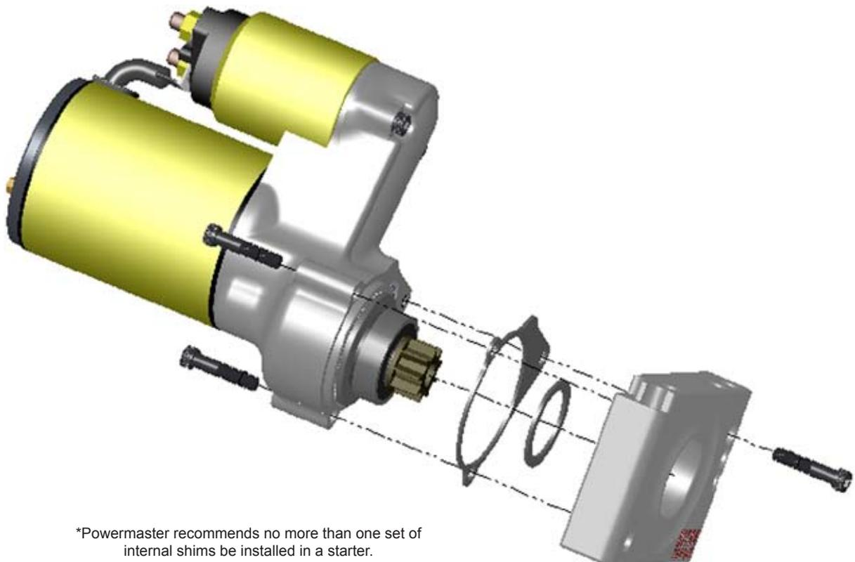
\*Powermaster recommends no more than one set of internal shims be installed in a starter.
