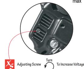
**WARNING: MAKE ADJUSTMENTS WITH ALL NONESSENTIAL VEHICLE ACCESSORIES OFF. ADJUSTING VOLTAGE WITH AMPLIFIERS, LIGHTS, OR OTHER HIGH AMPERAGE ACCESSORIES ON CAN RESULT IN DANGEROUSLY HIGH VOLTAGE WHEN ACCESSORIES ARE THEN SWITCHED OFF.**
