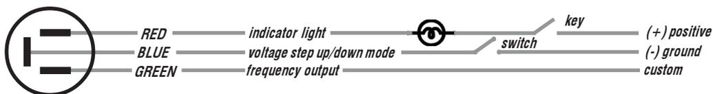
**INDICATOR LIGHT-** This is an output for a NO CHARGE indicator light. When this feature is utilized, a light will be illuminated when the key is in the run position and the alternator is not charging. The light will not illuminate when the engine is running and the alternator is charging.
